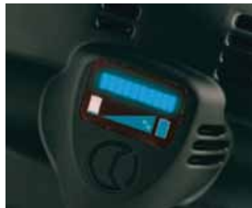
Battery Condition Display
