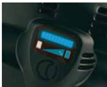
Battery Condition Display
